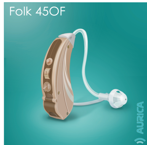
Digital 4-channels Hearing Aid with 5 memories for mild and moderate losses
